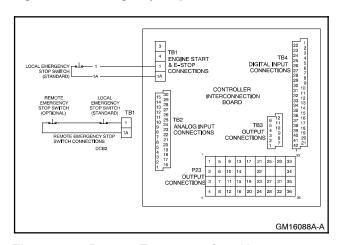
Figure 6-15 Remote Emergency Stop Kit Connections
